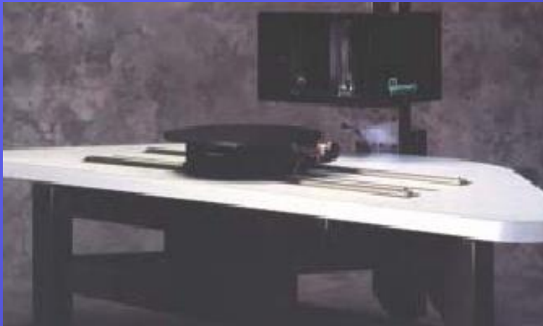
Laserski triangulacioni skener Cyberware MS 3030
